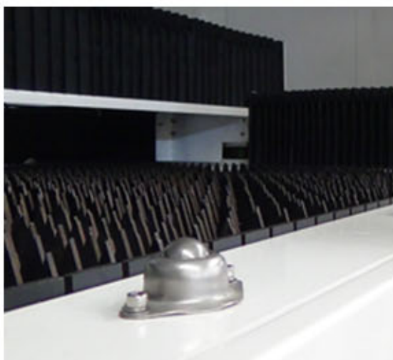
All around design with ball bearing, easy to edge feeding.
